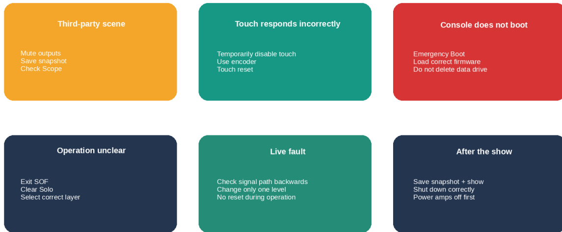
Figure 17: Fallback principles for typical faults. Original StageAID illustration.
